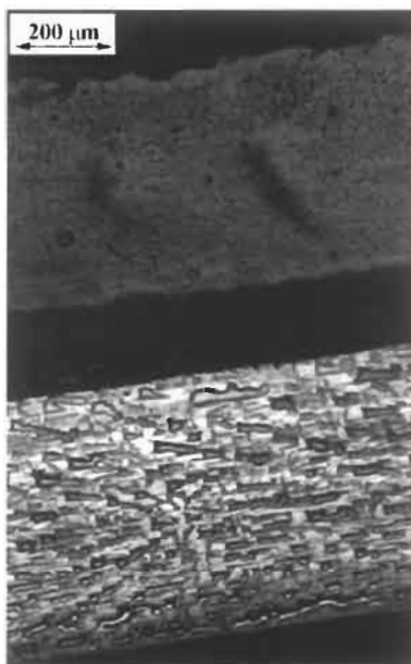
Fig. 11. The surfaces and edges of 600 \mu\text{m} wide \text{Fe}_{75}\text{B}_{15}\text{Si}_{10} ribbon produced on a Cu wheel. The lower half shows the side that was in contact with the wheel and the upper half the side that was in contact with the air. The diameter of the crucible orifice was 0.45 mm and the pressure needed to eject the liquid alloy was 0.4 \times 10^5 Pa. The Cu-wheel of 300 mm diameter turned with 1200 rpm.
